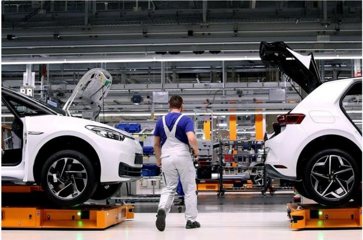
A Volkswagen assembly line producing the Volkswagen ID.3 electric car.
