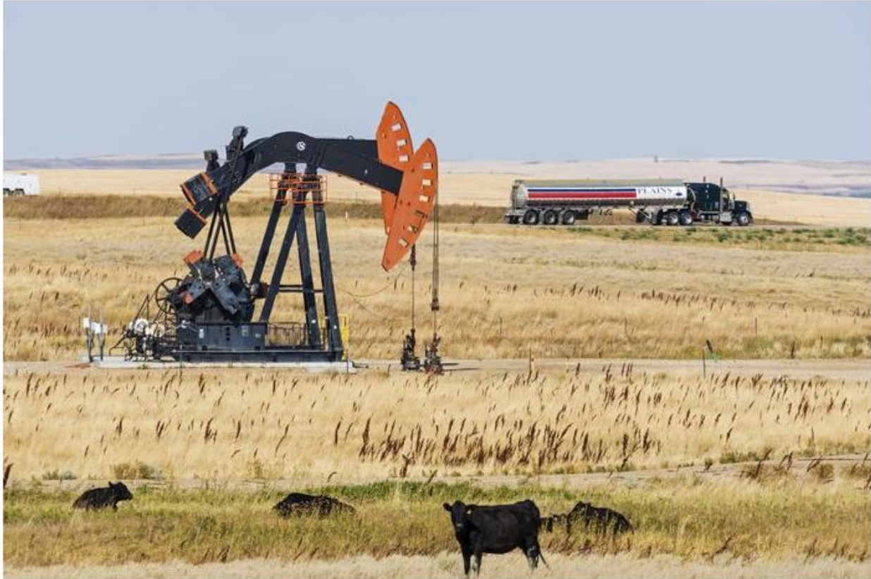
Oilfield pump jacks in North Dakota draw crude oil from a well in the Bakken Formation.
