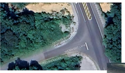
This project will reconstruct and resurface 4,500 feet of Port Authority Road, widen the entrance at KY 93 and add two-foot gravel shoulders. A full asphalt overlay is necessary, and a widened entrance and shoulders will improve turning radius for commercial trucks.
