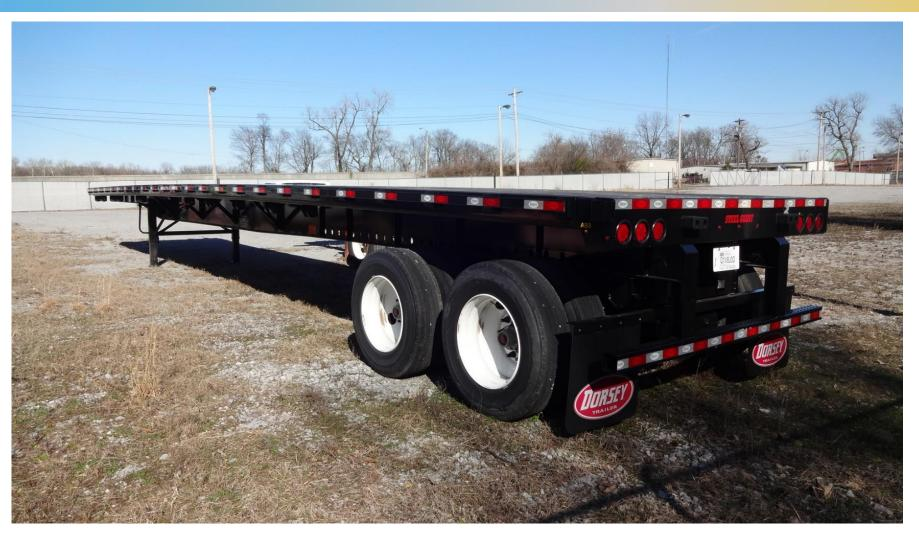
Project purchased a 48foot, spring slider, steel chassis flatbed trailer to replace rented trailer.
