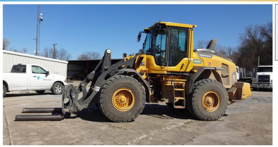
Project replaced wheel loader from 2003 that had become increasing difficult to maintain due to its age. Wheeled Loader used to load and unload bulk materials to truck once unloaded from barges.
