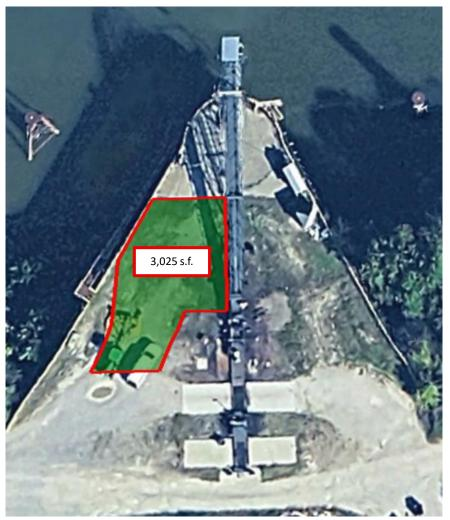
This project will construct a 3,025 square foot concrete pad 12" deep with rebar mats to provide a durable surface to allow semi-truck access and allow for efficient and environmentally safe cleanup of spillage.
