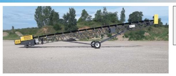
Project will purchase Triple Stack Portable Transfer Conveyor, Large Wheel Loader, and Radial Stacker to allow Riverport to continue current operations consisting of loading coal ash from the adjacent rail line facility. Also allow expansion of operations to include agricultural transport.
