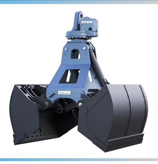
The proposed project would replace the current 4.5 cu/yd bucket with a 3.5 cu/yd bucket. A performance study found the material handler is currently operating beyond its designed hydraulic lifting capacity. A smaller bucket would allow machine to operate within its design parameters throughout unloading cycle range, which would reduce barge unloading time, unscheduled downtime and maintenance costs.
