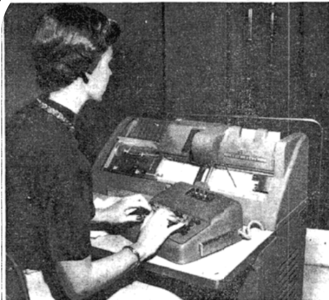
An electronic calculator produced by the International Business Machines Corporation was demonstrated yesterday in a new role: translating Russian phrases into English. The device has a "vocabulary" of 250 Russian words and can be adapted to other languages. Miss Marilyn Polle "types" Russian phrases on I. B. M. punch cards that are fed into the machine.
