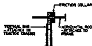
FIGURE W-18—Method of measuring instantaneous deflection.
